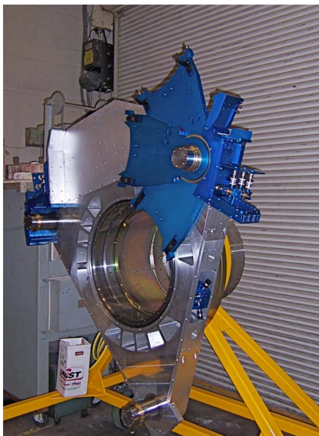
Figure 1: Major components of ODI's instrument support package are assembled on the instrument rotator simulator cart (yellow). The blue-colored parts will hold a third of the filter exchange mechanism. Three swing arms are visible: One is positioned in the beam, one out of the beam, and the outermost is in a position where the filter could be exchanged.
