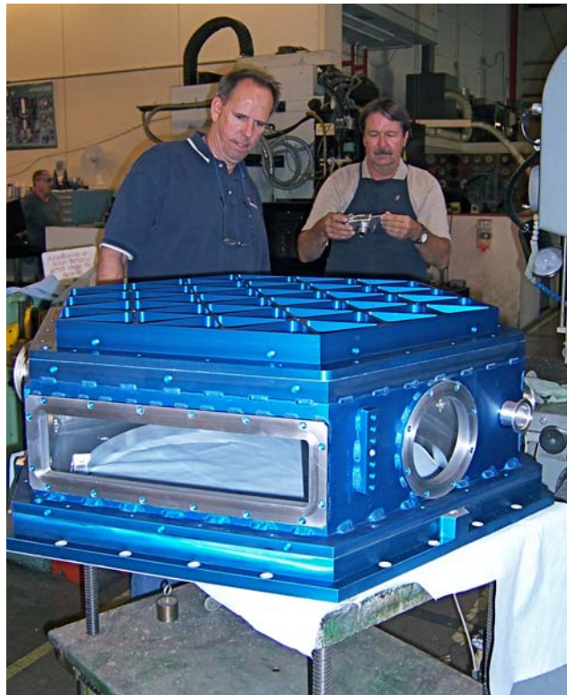
Figure 2: Gary Muller and Roger Repp inspect the ODI dewar shell. The CCD flex-circuit interface plate will mount on the large rectangular opening. One of the four cryo-coolers will be mounted to the large round opening at the right.
