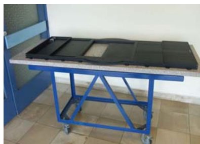
Figure 4: The Bonn Shutter for ODI during assembly. The two-blade design will allow linear exposures ranging from tens of milliseconds to hours with homogeneous illumination of the focal plane.
