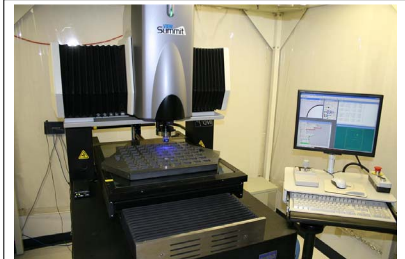
Figure 11. The VIEW Summit 600 coordinate measuring machine with the ODI SiC base plate under initial test. The flatness was measured to be about 10 \mu\text{m} peak-valley, as received.
