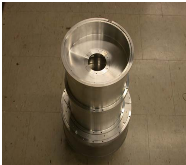
Figure 1: The WHIRC optical bench assembly fitted to the precision optical surface on top of the WHIRC dewar. This optical bench will be coated with Z306 black paint in the next and final manufacturing step.
