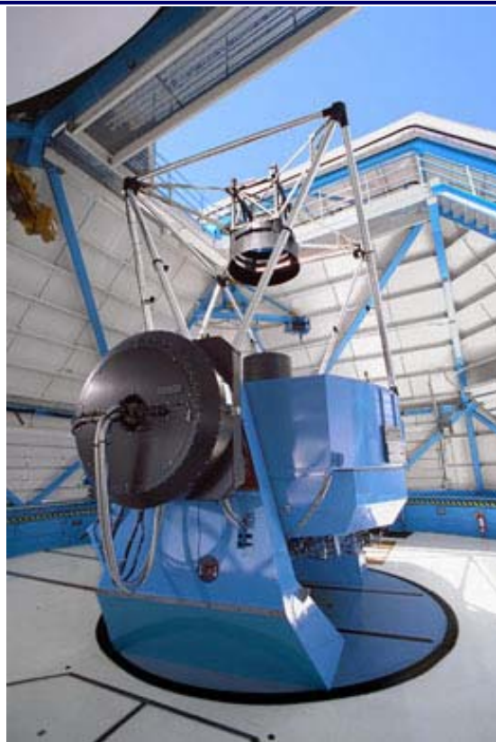
Figure 2: The WIYN 3.5-meter telescope showing the HYDRA Multi-fiber spectrograph front end attached to the side port. The metal cable coming from the instrument contains the fiber bundle that is routed to the telescope basement and connects to the bench mounted spectrograph.
