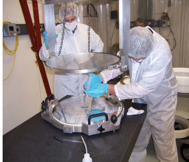
Test of the ADC bonding process with dummy wedges.
