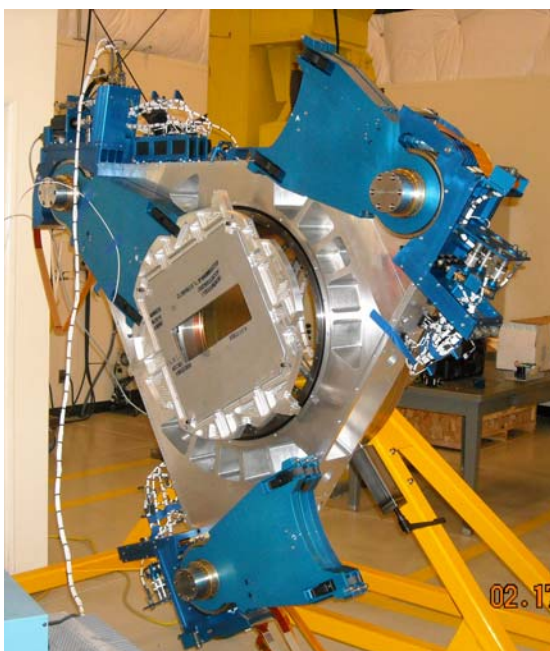
Figure 2: One filter swing arm is fully motorized. A filter change takes ~30 seconds.
