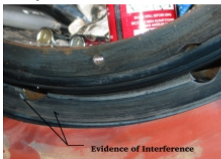
Figure 2: The mechanical interference is shown as light circular streaks which are integral to the fork and pillow block assembly.
