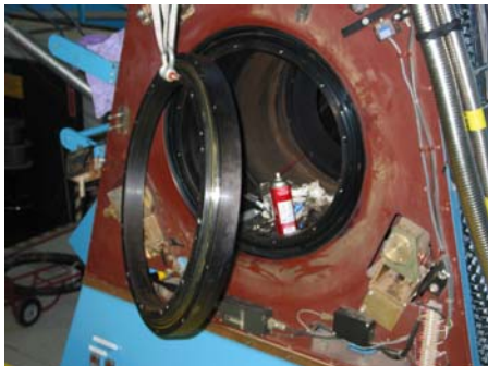
Figure 1: WNIR bearing is shown as it was removed from the telescope mount.
