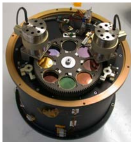
Figure 1: Filter wheel mechanism with filters installed.
