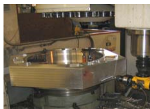
Figure 2: The ADC housing on the Hurco CNC machine being drilled with a newly acquired right angle boring head. Without this boring head, this drilling operation would have to be manually drilled on another machine. Credit: G. Muller.
