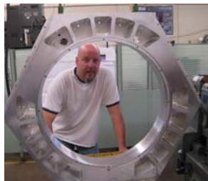
Figure 1: Instrument maker, Ron Harris, standing behind the aluminum Atmospheric Dispersion Compensator (ADC) housing (Part Number ODI-ME-02-1037). Three triangular shaped outrigger blocks will bolt to the housing to form the main structural component to which filter mechanisms and axles, ADC cells, and dewar will mount. When complete the housing will weigh 170 lbs
