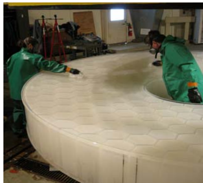
Figure 1: Final acid wash of primary mirror.
