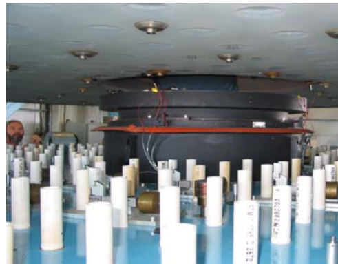
Figure 2: Primary being lowered onto the mirror cell.
