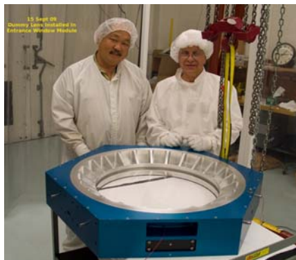
Figure 2: Ken Don and Bill Ditsler mount the test dewar window into the entrance window module.
