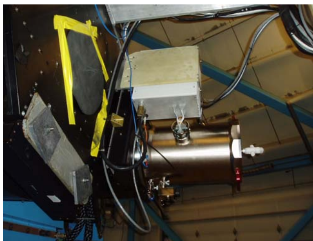
Figure 1: WHIRC mounted on the WIYN Tip-Tilt Module port.
