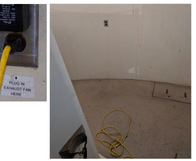
vi) **turn on the power strip for camera** by the northern platform screw pillar. Red LED will light to indicate it is on.
