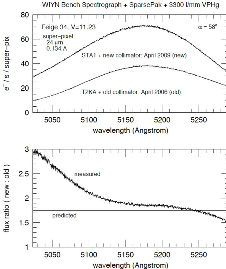
Figure 13. A comparison of the system throughput before and after the Bench Spectrograph upgrade. The top panel shows the flux as a function of wavelength, while the bottom panel shows the flux ratio, also as a function of wavelength.
