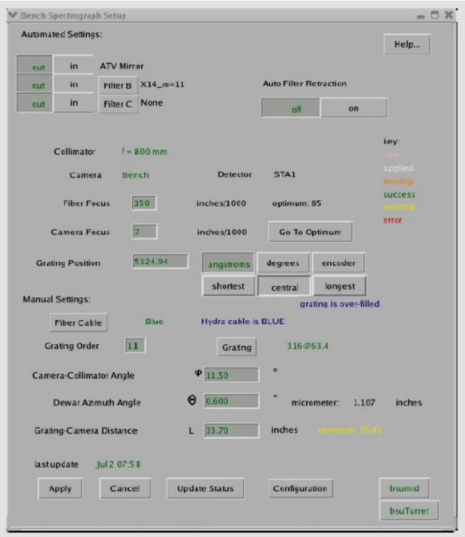
Figure 8. The new setup GUI for the Bench Spectrograph. In addition to duplicating the capability of the former GUI, a color-coded status reporting system was installed (color key is visible on the right about a quarter of the way down), and two status buttons were added for the two processes that run the Bench (see bottom right corner.)
