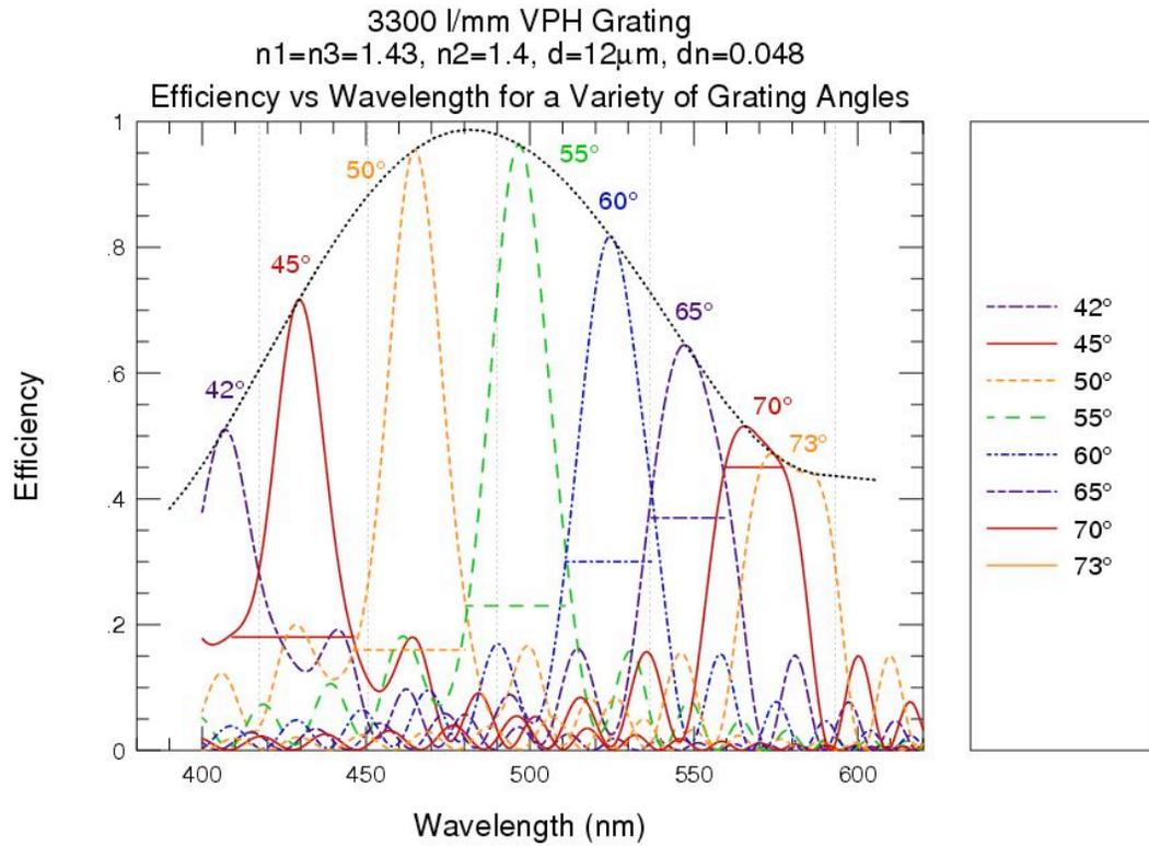
Figure 2. Predicted relative efficiencies for the 3300 VPH for several grating angles.
