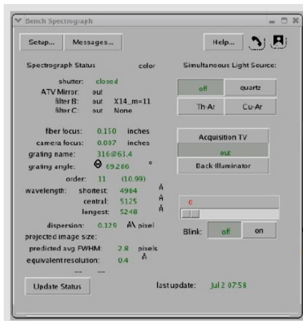
Figure 9. The new Bench calibration and object acquisition GUI. This allows the observer to control the various calibration lamps (see right, about one quarter way down), as well as insert either the acquisition TV or back illuminator and control the illumination of either to aide in target acquisition (see middle and lower quarter right). The left side reports the details of the current grating configuration.
