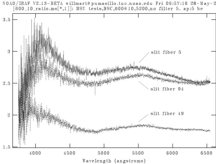
Figure 12. A comparison of the relative throughput improvement before and after the Bench Spectrograph upgrade as a function of wavelength for three red Hydra fibers. Fiber 49 is near the center of the fiber pseudo-slit, while fibers 5 and 94 are near the ends.
