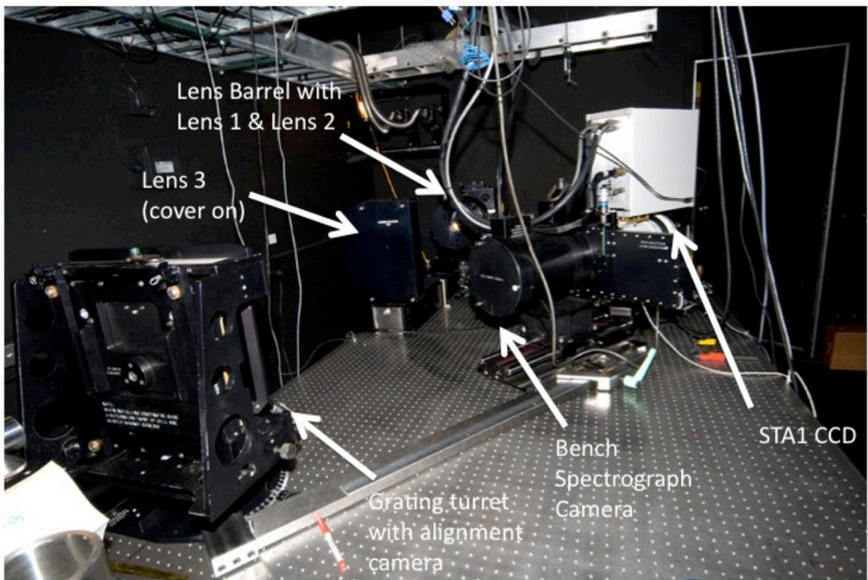
Figure 6. New collimator and most other major components on optical bench during the alignment procedure. Not shown are the fiber foot, the ATV, or the BSC rear lens element.
