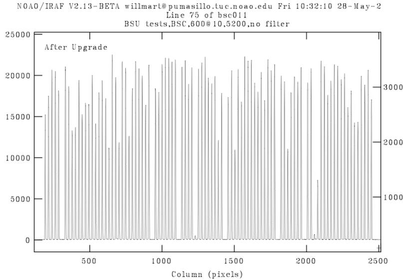
Figure 11. A cross-cut of the fibers in the spatial direction after the upgrade. The inverted “u” shape is gone. Remaining variations from fiber to fiber are due to the quality of the prism attached to the input end of the fiber and inherent stresses in each fiber. Gaps represent broken fibers.
