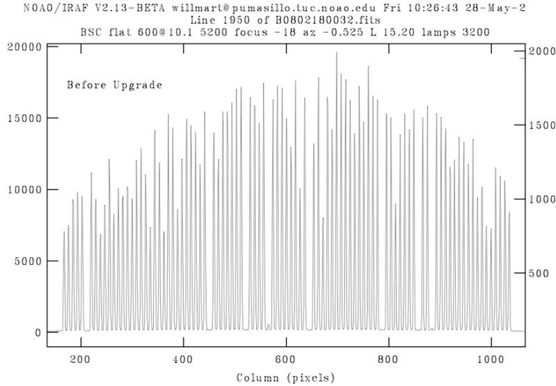
Figure 10. A cross-cut of the fibers in the spatial direction before the upgrade. The vignetting in the spatial direction produced the inverted “u” shape in the overall response of the fibers. Other variations from fiber to fiber are due to the quality of the prism attached to the input end of the fiber and inherent stresses in each fiber. Gaps represent broken fibers.
