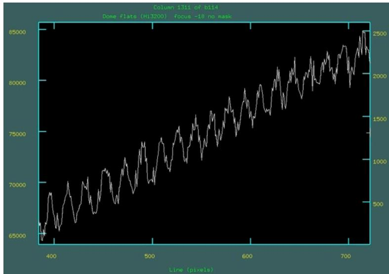
Figure 1. A sample of fringing for STA1 at around 7500  $\text{\AA}$ . Data are from a single column of a quartz lamp flatfield exposure and have been overscan subtracted.
