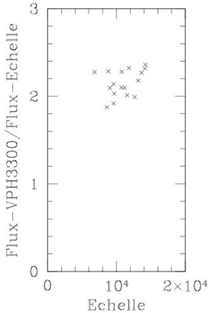
Figure 4. The measured flux ratios for ~20 lines for the 3300 l/mm VPH grating and the 316@63° echelle at 5130 Å ( $\alpha=57.8$  degrees). The 3300 l/mm grating is about twice as efficient as the echelle in this setup.
