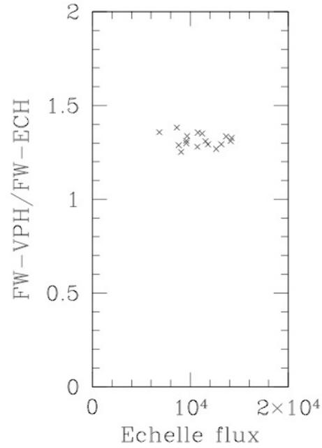
Figure 3. The measured ratios of line widths in the direction of dispersion for the 3300 l/mm VPH grating and the 316@63° echelle at 5130 Å ( $\alpha=57.8$  degrees). The anamorphic demagnification of the echelle narrows the lines about 30% compared to the VPH.
