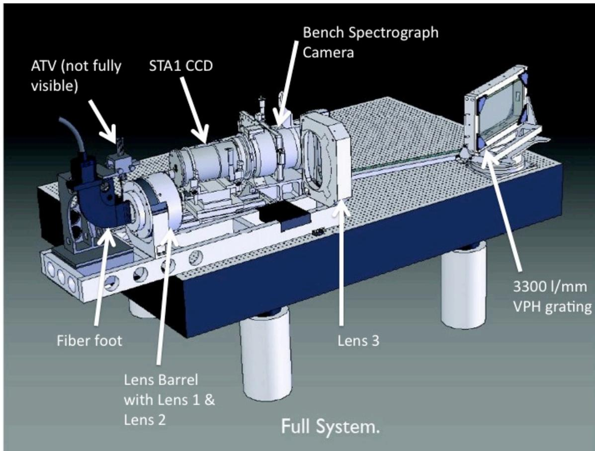
Figure 5. Rendering of the upgraded Bench Spectrograph. Not shown is the electronics box that mounts to the STA1 CCD or the BSC rear element.
