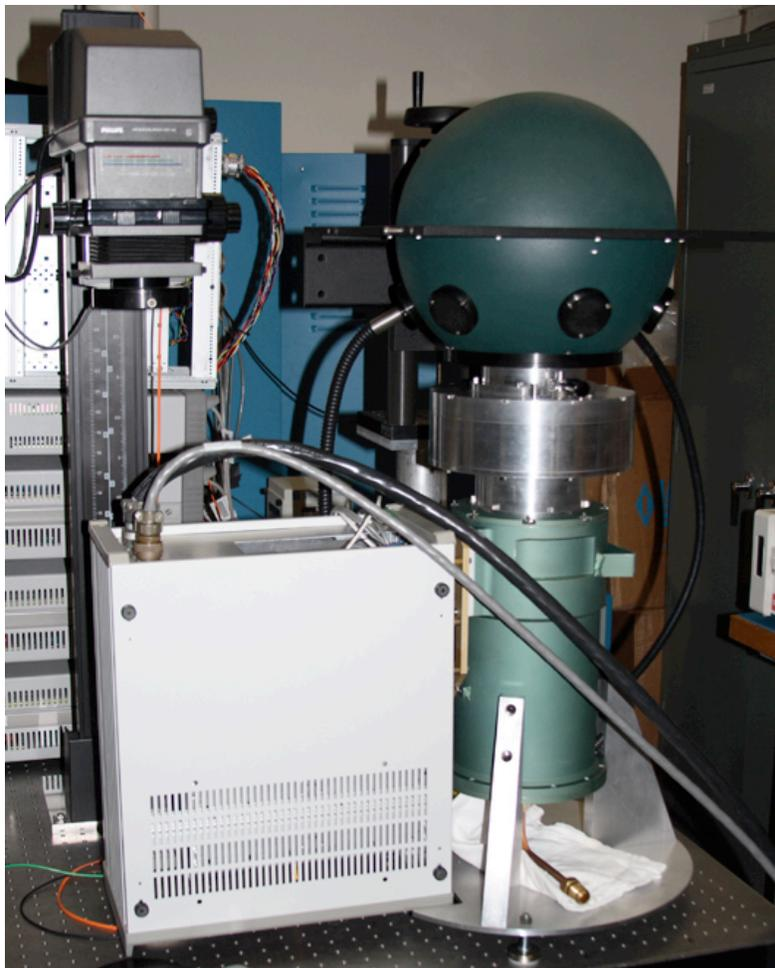
Figure 1 - Lab setup for the STA1042 tests: The test dewar is connected to the integrating sphere and the image projector is visible to the left. The MONSOON DHE is the white box, the UGD is to the right of the DHE, the test interface “snout” is the bright aluminum interface between the dewar and I-sphere.
